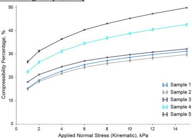
Sample 5 was the most compressible of the materials, indicating that if stored in large quantities, it would be more susceptible to consolidation. High Compressibility indicates that a powder entrains a greater proportion of air within its bulk, which is a property typically associated with more cohesive, inefficiently packed powders.
