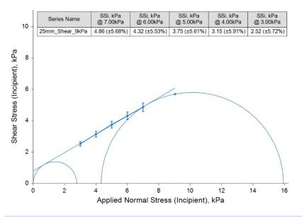
Minimal differentiation was observed between the five samples. Near identical Shear Stress values were generated (RSD <6%).
