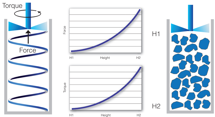
Torque and Force are measured simultaneously as the blade moves down a helical path through the powder
